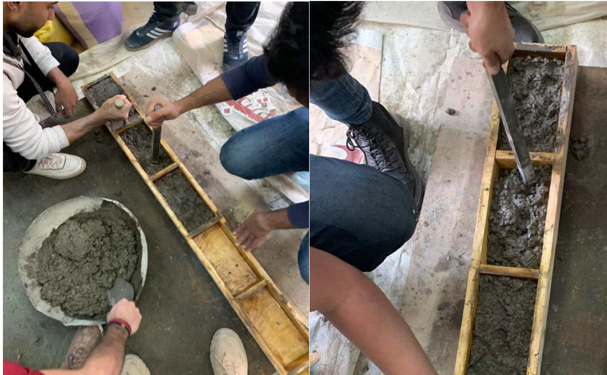
Figure 3.36 compaction the concrete
