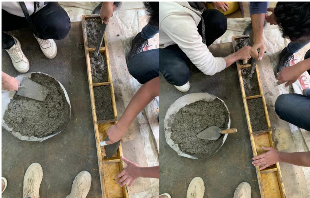
Figure 3.35 placing the concrete.
