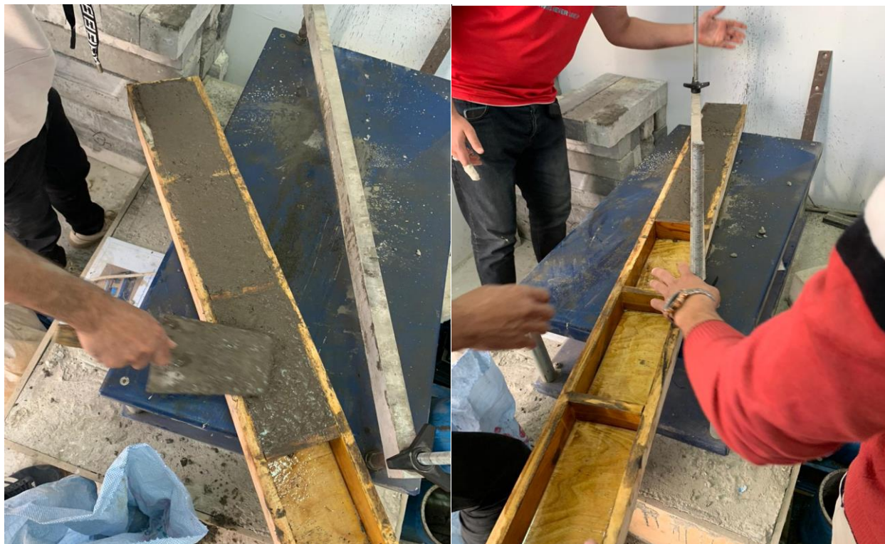
Figure 3.37 shaking to compact the concrete.
